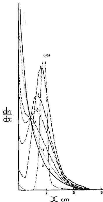
Fig. 3. Curves obtained during a D.O.E. experiment on rabbit serum performed concurrently with the B.S.A. run (Fig. 2). The numbers denote the time intervals in days. Equilibrium was reached after approx. 21 days. The ordinates are the refractive index gradients. —, equilibrium curve.
